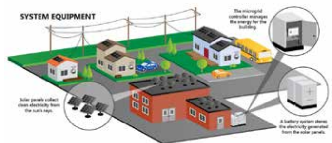
Figure 59. How a microgrid works. Source: Franklinwh.com
