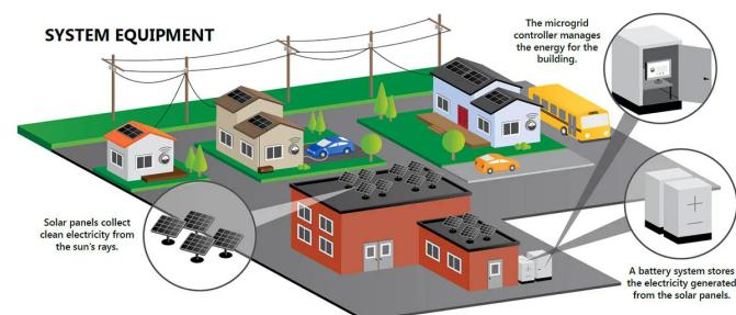
Figure 59. How a microgrid works. Source: Franklinwh.com
