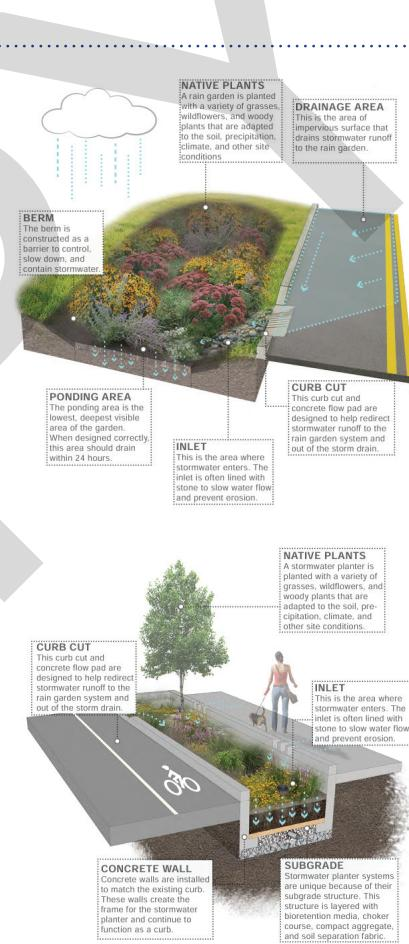
**Figure 49.** Examples of small-scale stormwater infrastructure, from NJ DEP’s Resilient Landscapes guidance document.
