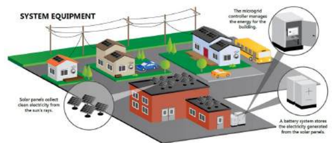
Figure 59. How a microgrid works. Source: Franklinwh.com
