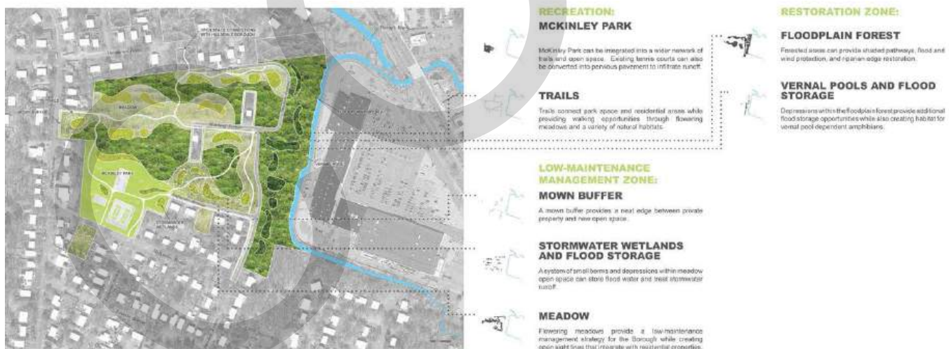
Figure 63. Resilient park designed to reduce harm from flooding. Credit: Rutgers Cooperative Extension, obtained from NJDEP's publication, Creating Flood-Resilient Landscapes.
